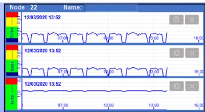
A set of Trend Charts give you a visualization of Vibration Axis and Temperature for each bound node. The charts update to a new device every 6 seconds. The indicator bar colors indicate state levels of the data, **Blue** – Noise Floor (Off), **Green** – Operating Zone, **Yellow** – Warning Zone and **Red** - Critical Zone. The Axis with the highest vibration sets the max scaling.
