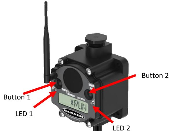
1. After the binding is started from Vibe-Sight, press the 2<sup>nd</sup> button 3 times to start binding.
