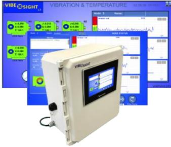
The VS700LTM is set up to monitor 6 different devices, whether they are motors, bearings, or machine assemblies. The default configuration uses the Banner Wireless Gateway (900 MHz FHSS radio) along with their wireless vibration nodes. Vibe-Sight Lt can be upgraded in groups of 6 up to a total of 18 Devices.
