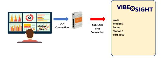
For this connection the external connection from Vibe-Sight needs to be to the WAN port on the Tosibox security Device.
