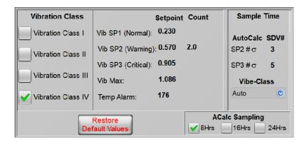
Use this section to Customize your vibration levels. Section 8. Determining Setpoints, discusses the Different Vibration Classes in depth. The setpoints are predefined by ISO standard, but you wished to make a custom class for your system you can modify "Globally" one or all Vibration Classes.
