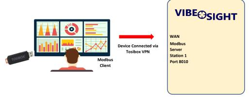
For this connection the external connection from Vibe-Sight needs to be to the WAN port on the Tosibox security Device.
