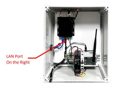
Using an Internet Browser connect to Tosibox's internal Webpage. Its IP address is 10.10.10.254 The Tosibox Password on Vibe-Sight is pre-configured to VS and the Password on the bottom. When you connect the following screen will display.
