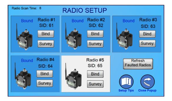
The Radio Setup Screen gives you a quick indication of Bound and Unbound Radios. There is also an indication of the scan time of the Master Radio for troubleshooting information.
