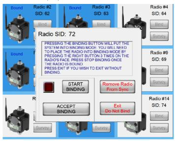
Press "Start Binding", the Binding indicator will turn Red to indicate that Binding has started. (Note, Binding is not allowed via Remote Connection)
