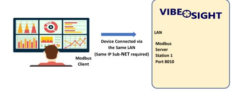
For this connection the external connection from **Vibe-Sight** needs to be the internal Lan connection from the switch, or make the second Network port on the cMT match the Plant Network Subnet and use it. **Vibe-Sight** will have to be changed to the same subnet or the second port on the cMT will need to be set up. (See Addendum 1). Note, on **Vibe-Sight**<sub>Lt</sub> you must use port 1 disconnecting it from Tosibox.
