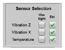
Starting with Vibe-Sight V2, you can now select whether your sensors for the device are connected via the Banner Wireless Nodes and are accessed from the Banner Gateway or come from external sources. If you Select Vibe-Sight (Int) the sensors will be the standard Banner Wireless sensors as normal.
