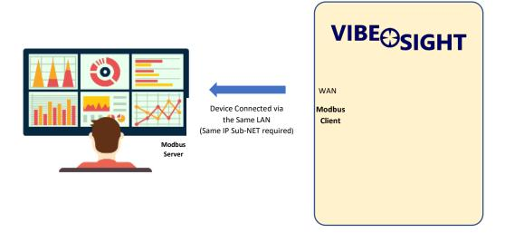
If your SCADA or MES Computer can be set up as a Modbus Server, the Vibe-Sight gateway can be setup as a Modbus Client. With this, the Data can be routed from the WAN port of Vibe-Sight past its firewall and through to the Server.
