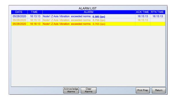
The Alarm Screen shows all Alarms on the System. Each node is represented by its Node Number, then the Alarm Condition with value are listed. Finally, the Acknowledgement time and the time the alarm returns to its normal condition are displayed. Color Code is as follows:
