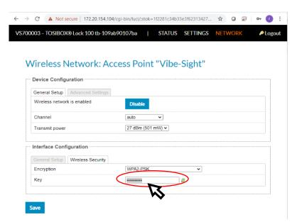
Set the Encryption type and then enter the password into the field marked Key. Hit Save. Your lock will restart and will connect to the Internet.
