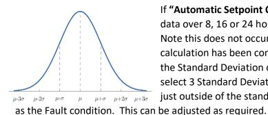
If "Automatic Setpoint Calculation" is selected we sample the data over 8, 16 or 24 hours of actual run time (8 is default). Note this does not occur until the Automatic Runtime calculation has been completed. When complete, we calculate the Standard Deviation of the Sample set. Then By default, we select 3 Standard Deviations as the Alarm Condition effectively just outside of the standard curve, and 5 Standard Deviations
