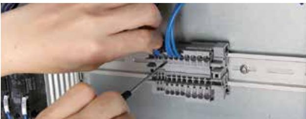
**BEFORE** One hand wiring with the other hand holding the screwdriver
