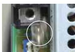
**BEFORE** The screw is loosened and dropped by vibration
