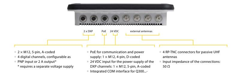
LNX/-WIN connection for the UHF DTM
