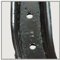
Mounting holes are present and completely punched out.
