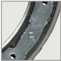
Text is positioned correctly relative to the position of the stamped holes.
