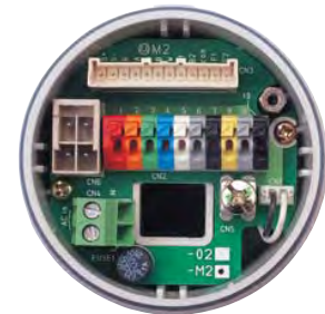
Color Coded Wiring Terminals
