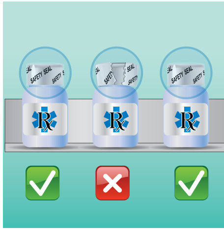
Verify tamperproof seal presence
