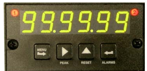
Laureate 6-digit timer, one of the software configurations of the 6-digit counter.
