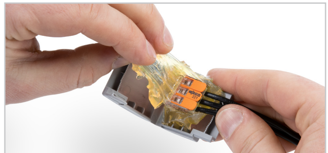
Open the Gelbox., remove gel from the connector, open the connector and connect new components to the cable
